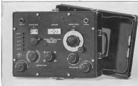
The TYPE 761-A Vibration Meter is used by builders of mechanical equipment to measure the magnitude of vibration as a step in its elimination.
